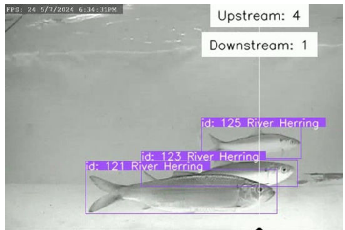
Annotated video frame showing a machine-learning algorithm identifying and counting river herring as they pass the camera and move upstream in the Coonamessett River (Photo courtesy of Dr. Zhongqi Chen, Woodwell Climate Research Center).
