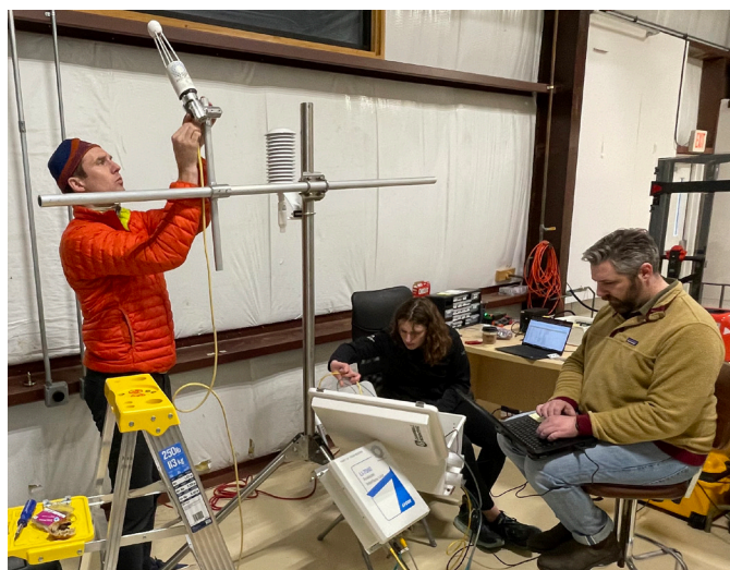
Kaj Lynøe, Dani Trangmoe, and Patrick Murphy prep eddy covariance tower equipment for field placement later in the spring. / photo by Kecy Kent
