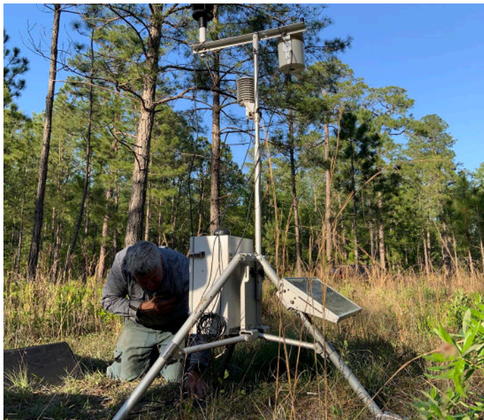
left: Joseph O'Brien from the U.S. Forest Service installs a meteorological station ahead of the prescribed burn. right: A timber rattlesnake, native to Georgia's pine forests. / photos by Joshua Rady
