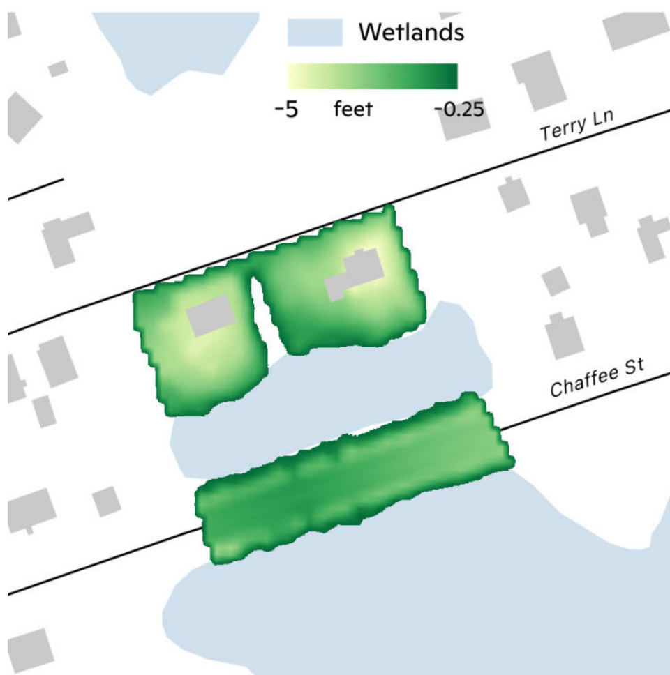
Figure 4: Elevation changes. The area shown has the elevation lowered to include flood model modifications. The two buildings shown in the elevation change would be removed in this model scenario.
