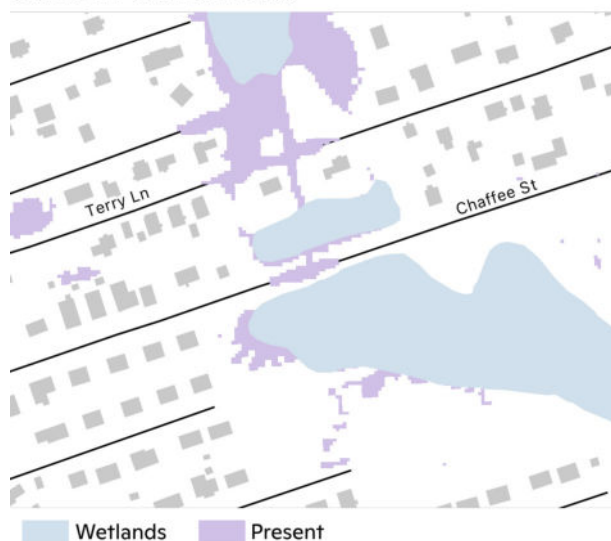
Figure 5: Present-Day and Future 100-Year Flood Modifications. The flood extent, quantified as having a depth of at least 0.5 ft (0.15 m), for New Bedford, MA. Current culverts are modeled on the left, and the right includes changes to the culverts and elevations. In this scenario, the two buildings in the wetland would be removed. The maximum extent for the 100-year pluvial/riverine flood is shown.
